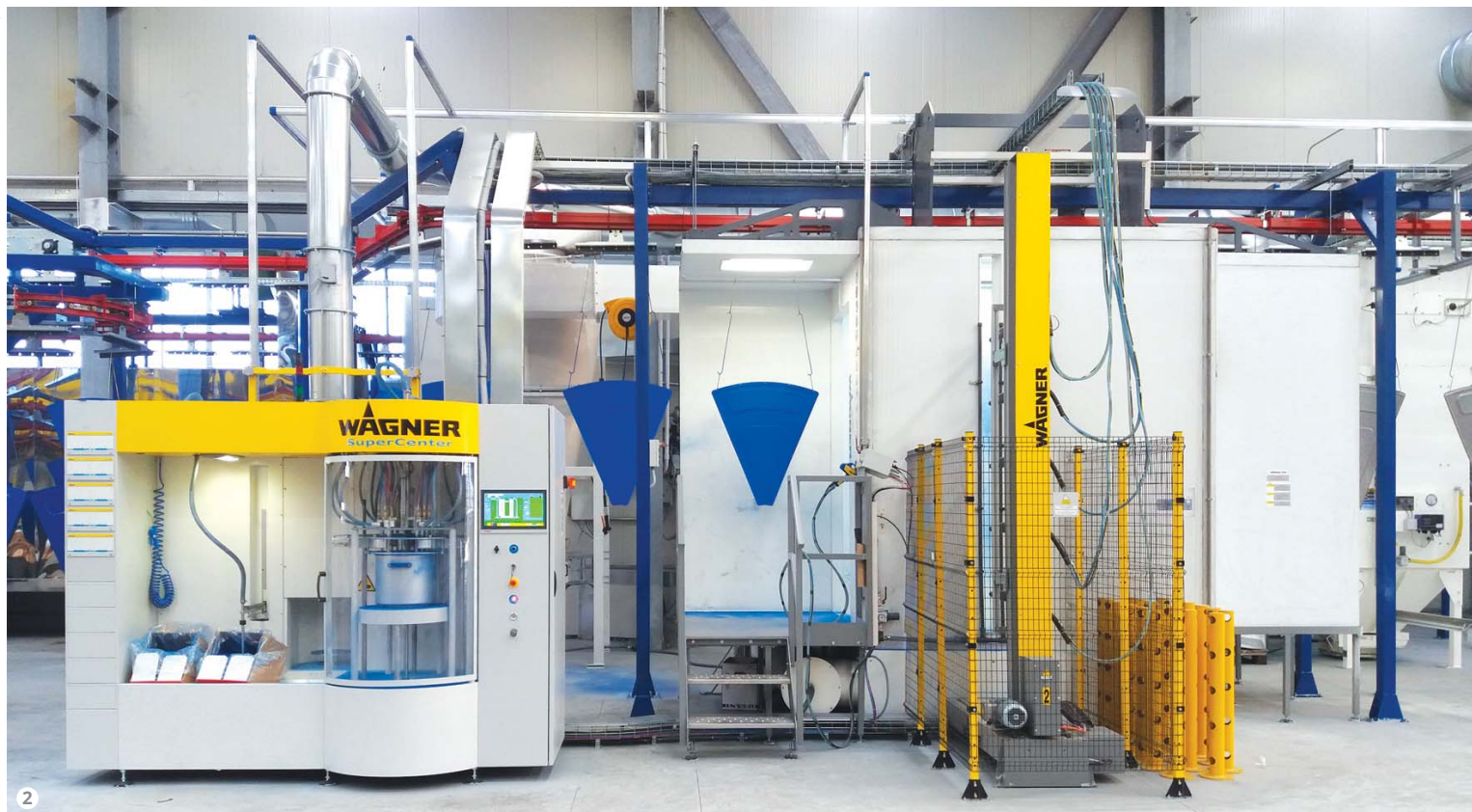
Figure 2: The Wagner SuperCenter automatic coating booth with a quick colour change system.
