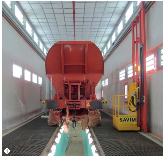
Figure 1: The coating booth becomes like a series of adjacent identical booths without any separation between them.
