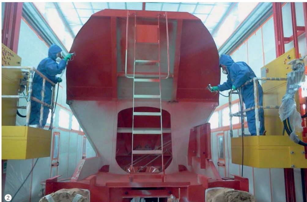
Figure 2: Each of these booths has an autonomous functioning, identical or different from the others. The PLC manages the cycle, whereas the operator only gives consent based on his position.
