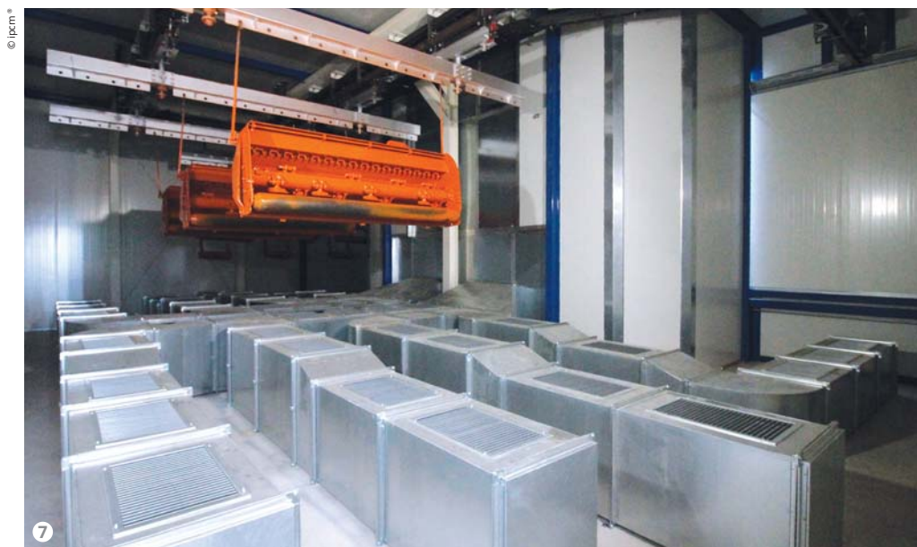
Figure 7: The curing stage in the direct fired furnace.
