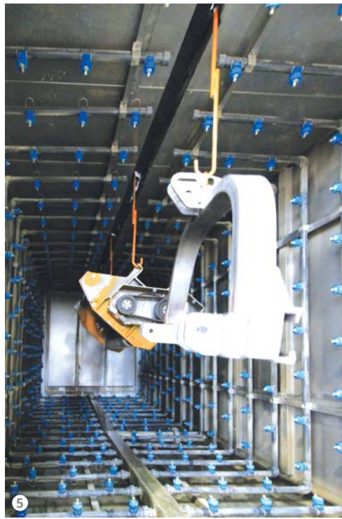
Figure 5: The 3-stage chemical pre-treatment process.
