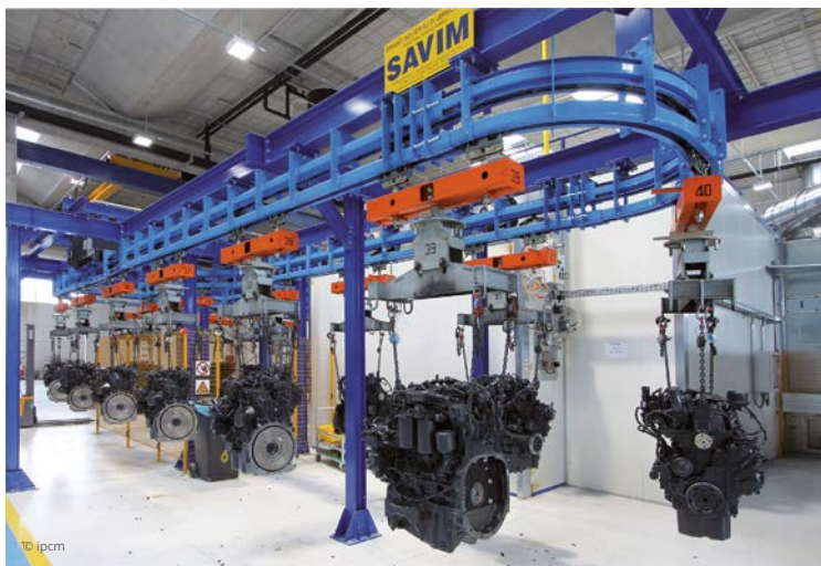
These painted engines leave the drying oven and head for the unloading station.
