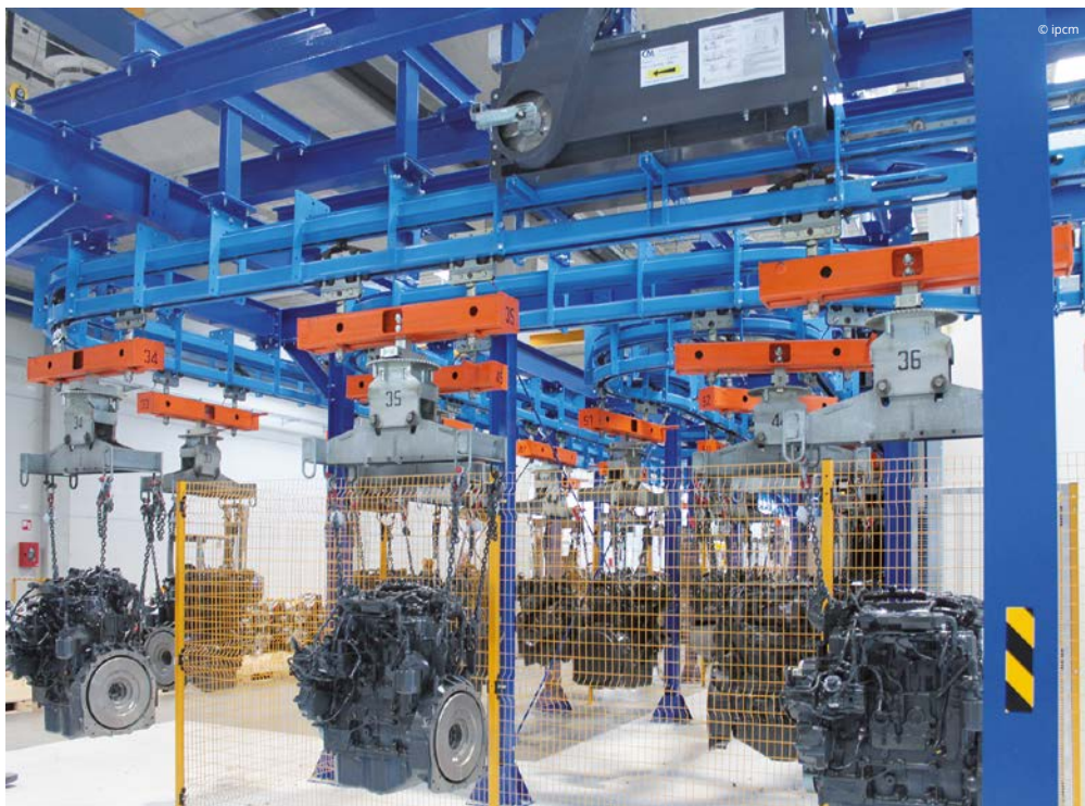
The XD45/59 step-by-step conveyor provided by CM Automazione houses up to 116 handling units equipped with a ring-gear idler swivel hook.
