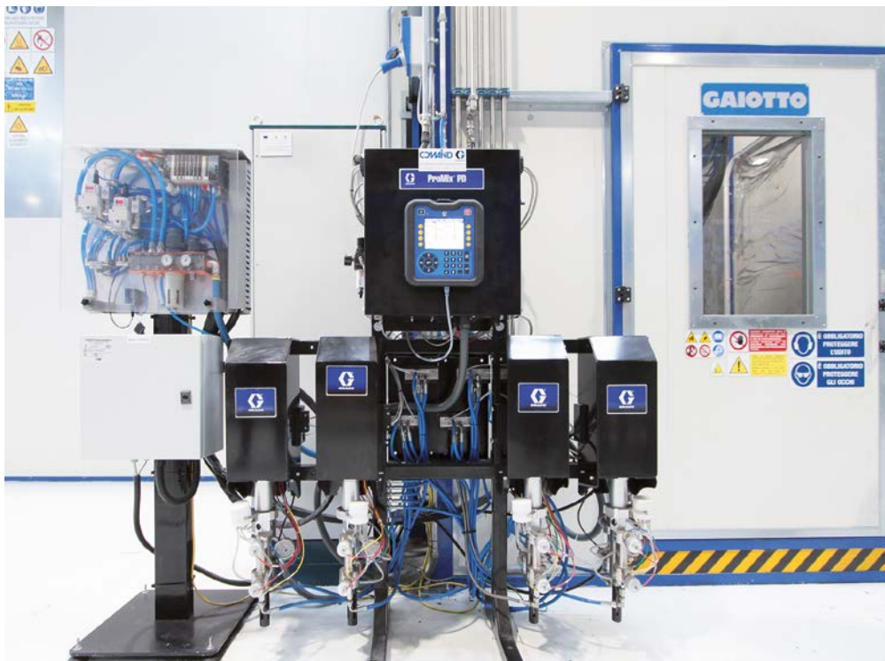
The Graco PD1K mixing machine with four separate pumps for each colour, installed by Comaind (San Giovanni Lupatoto, Verona).
