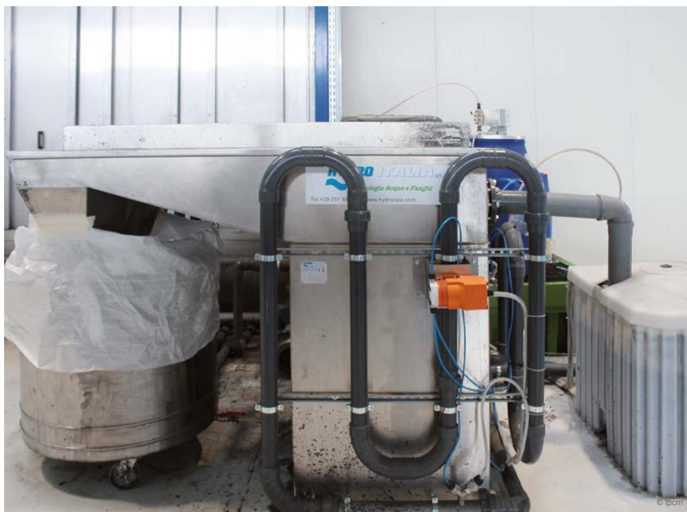
Hydro Italia's sludge separator treating the water coming from the coating booth's overspray collection curtains.
