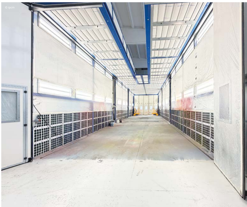
The Savim Europe booth in its entirety: it is 24 metres long and 6 metres wide.
