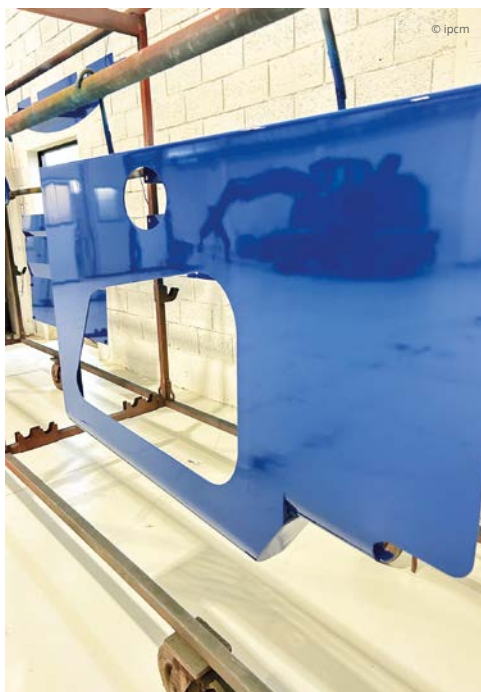
A part of a coated handler's bodywork and the inside of the booth: the largest parts to be treated are lowered from above using an overhead crane.
