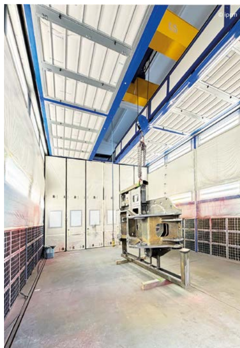
A part of a coated handler's bodywork and the inside of the booth: the largest parts to be treated are lowered from above using an overhead crane.
